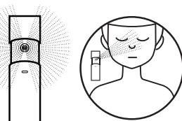
**D3 (NANO MIST DIFFUSER) TECHNICAL SPECS:** Rechargeable: via Micro USB / Micro USB cable included / Operating current: 350±50mA / Max power: <1.8W Static power consumption: <70uA / Automatic safety shutdown after 50 sec. / Tank capacity: 9 ml / 0.30 fl.oz
